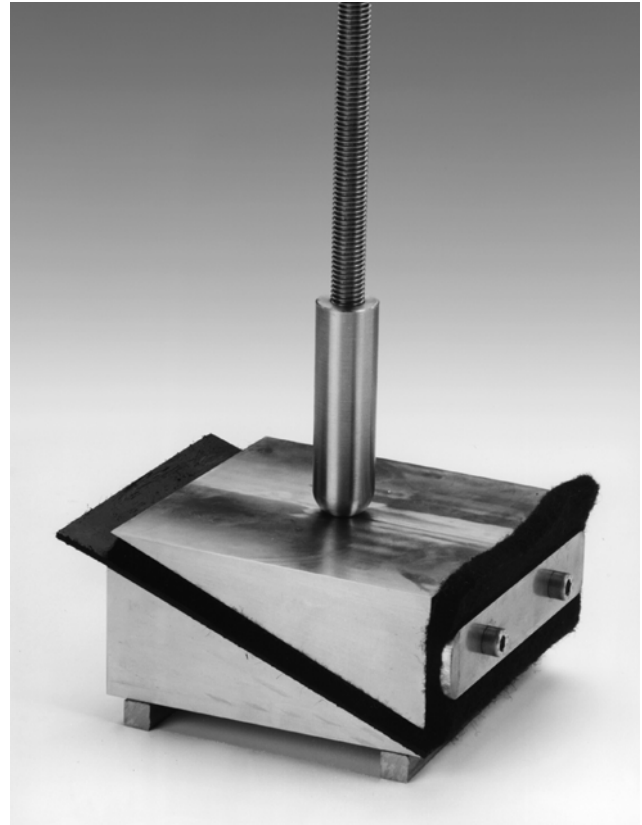
Figure 3 Specimen holder mounted with textured GM specimen and geotextile specimens as friction partner
