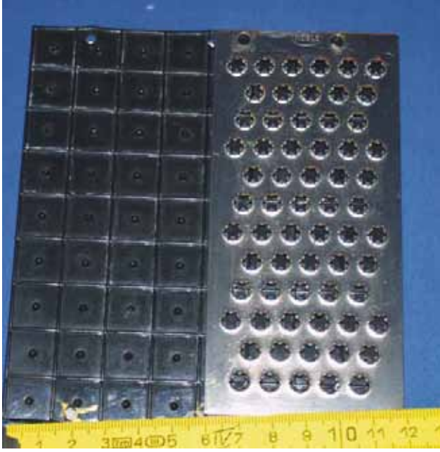
Figure 4 Two textured friction partners, which were mounted onto the wedges ensuring high friction and firm contact to GCLs or GCDs
