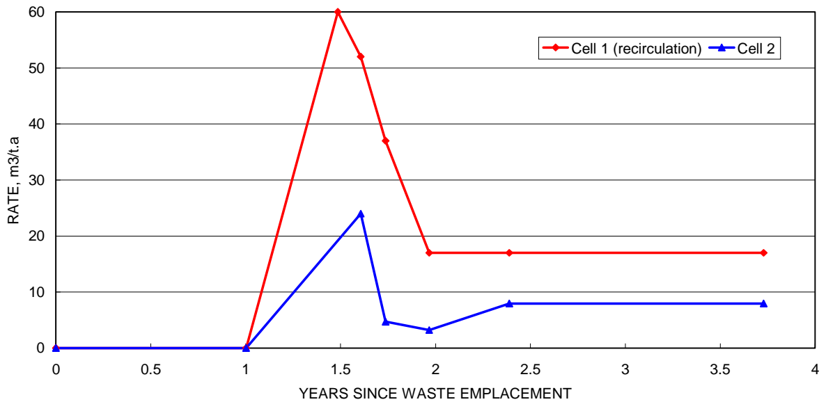
Figure 5. Cumulative gas flow at the Landfill 2000 test cells
