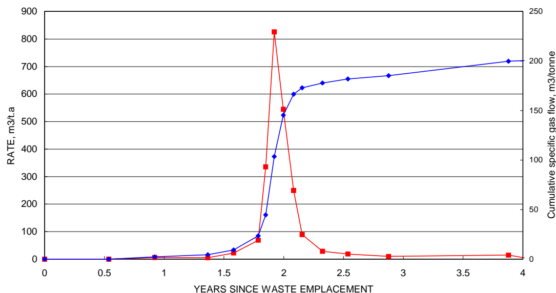
Figure 3. Gas generation in an optimised small scale reactor (Beaven, 1996)
